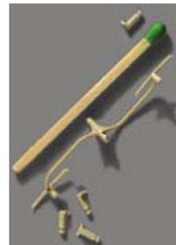
These switch pins are an example of how micromolding saves time and materials. They have the same weight, 0.017 g. But the ones on the left, made by conventional molding, required a shot weight of 0.23 g, a sprue/runner weight of 0.165 g, and a cycle time of 6.3 sec. Whereas the ones on the right, made by micromolding, required a shot weight of 0.109 g, a sprue/runner weight of 0.044 g, and a cycle time of 2.7 sec.
